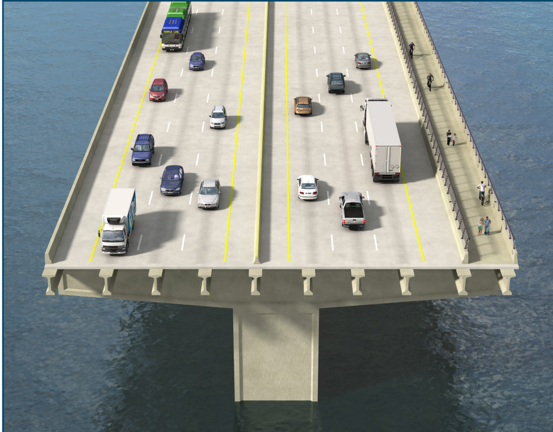
Figure 3-34 Recommended Preferred Alternative 4A Bridge Cross Section
