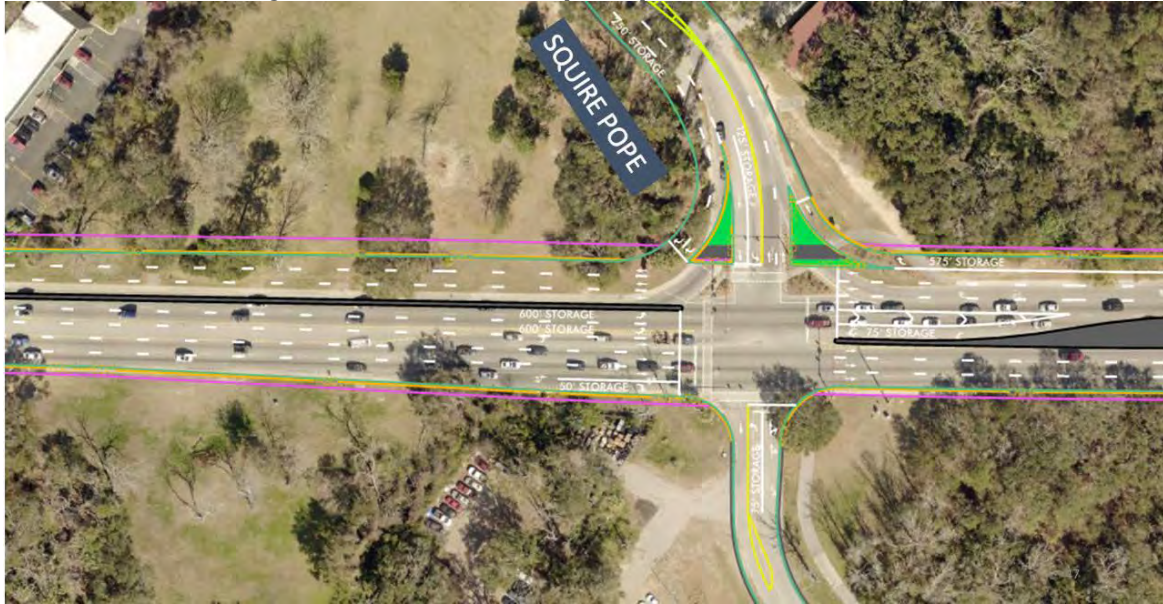
Figure 21 – Maximize Lanes at Spanish Wells Road Intersection Concept
