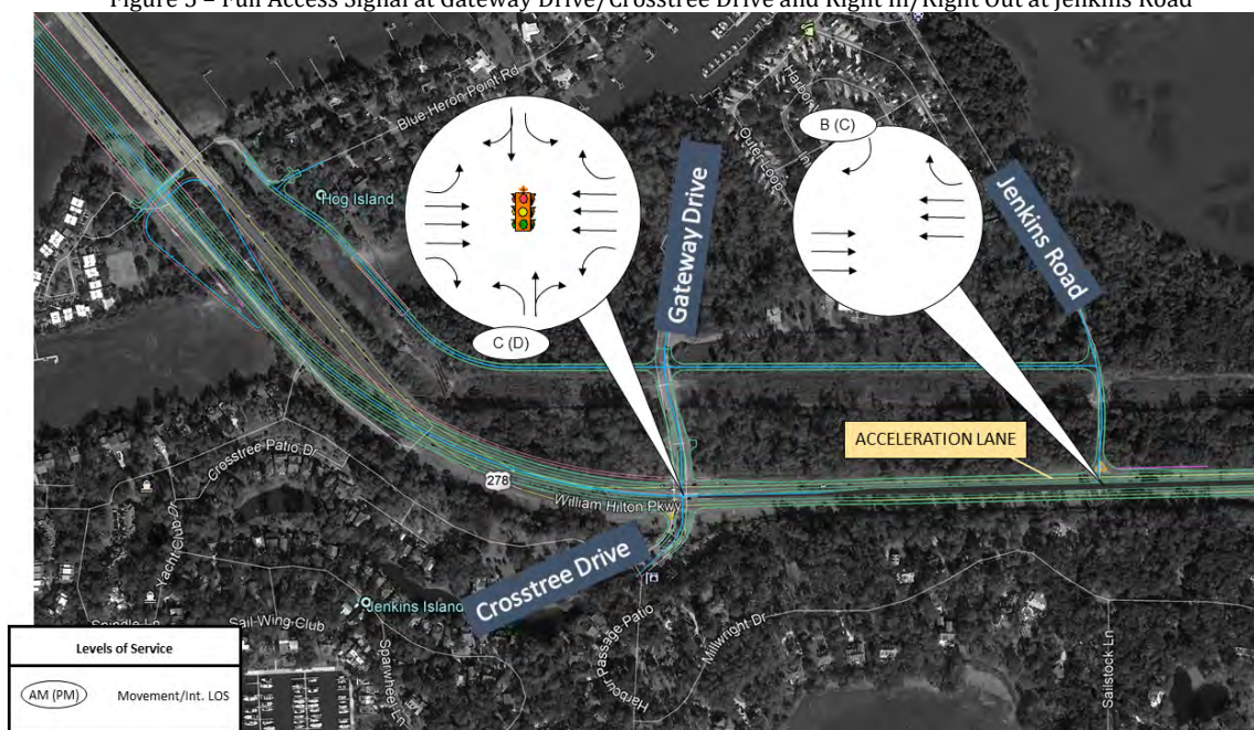
Figure 5 – Full Access Signal at Gateway Drive/Crosstree Drive and Right In/Right Out at Jenkins Road
