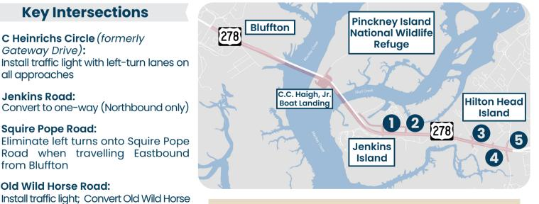
For access to the PINWR and the C.C. Haigh Jr. Boat Landing, Alternative 4A proposes a new right-in/right-out type of interchange.
