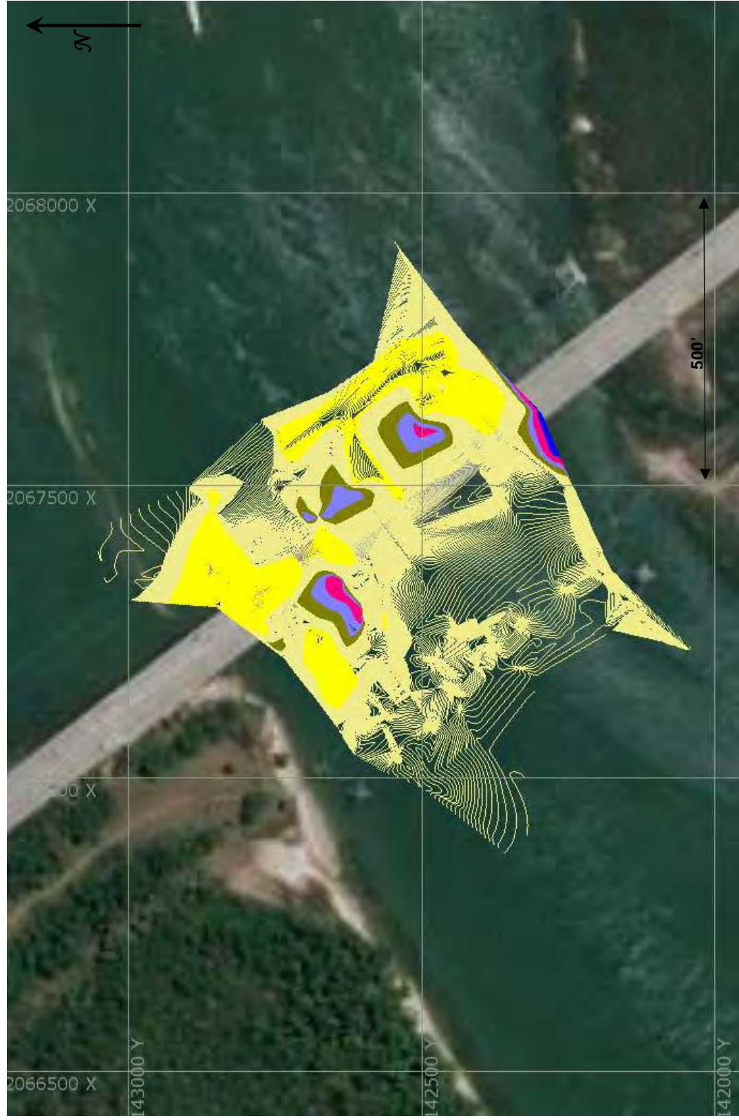
Figure 9. Magnetic Contours at 10 nT (gamma) Intervals of Skull Creek Project Area overlaid on Aerial Photograph
